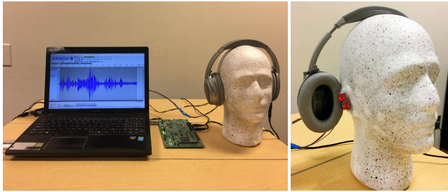
Figure 11: MUTE+Passive : (a) Bose headphone on the 3D head model, with DSP output connected to the headset. (b) The measurement microphone inside the ear, and the reference microphone nearby.
